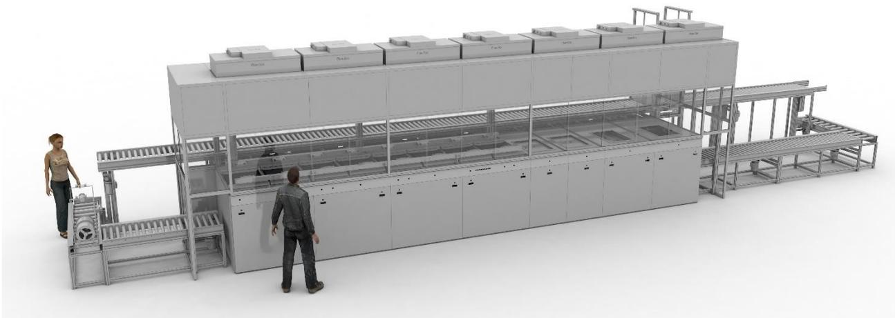
The enclosure comprises integral filter systems to support cleaning under cleanroom conditions.
