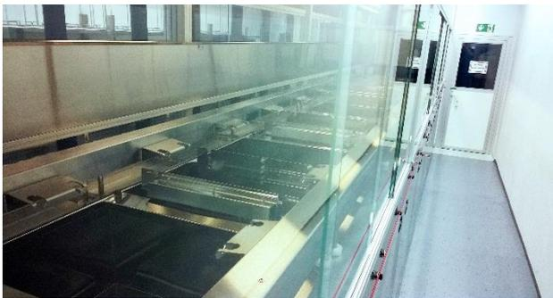
The cleaning system comprises a total of 13 stations. All process sequences and parameters as well as equipment functions are automatically monitored, logged and documented on a continuous basis.
